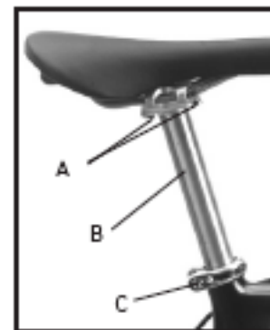
Figure 16- Seatpost parts A- Seat fixing bolts B- Seatpost C- Seatpost binder bolt
