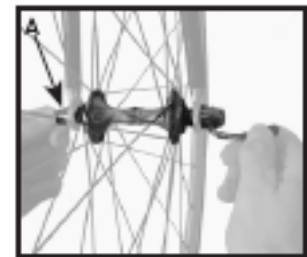
Figure 33- Tighten nut A- Adjusting nut
