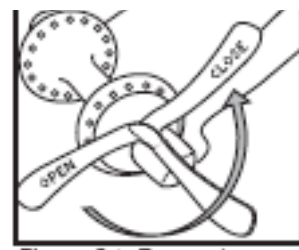
Figure 34- Proper lever throw
