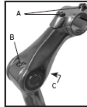
Figure 12- Adjustable-rise quill stem A- Handlebar clamp bolts B- Stem expander bolt C- Angle adjusting bolt
